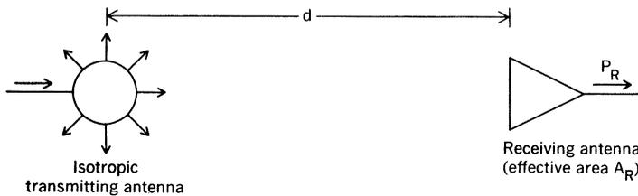
FIGURE 15. Relation between the gain and the effective area of an antenna.
