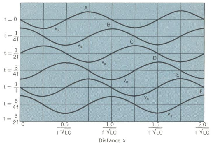
FIGURE 8. Line voltage  $v_x$  vs. distance  $x$  along the line.
