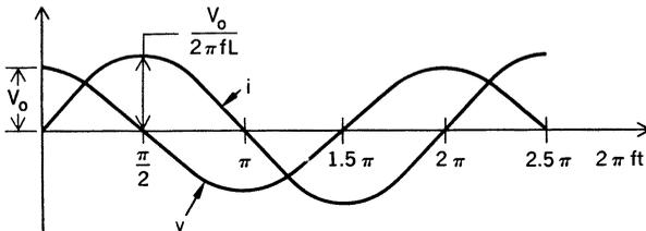
FIGURE 3. Voltage ( $v$ ) and current ( $i$ ) vs.  $2\pi ft$  for inductive circuit of Fig. 2.
