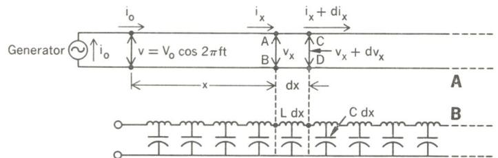
FIGURE 7. A—Long uniform transmission line. B—Equivalent lumped-circuit line.
