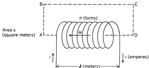
FIGURE 1. Long coil of wire with direct-current flow.
