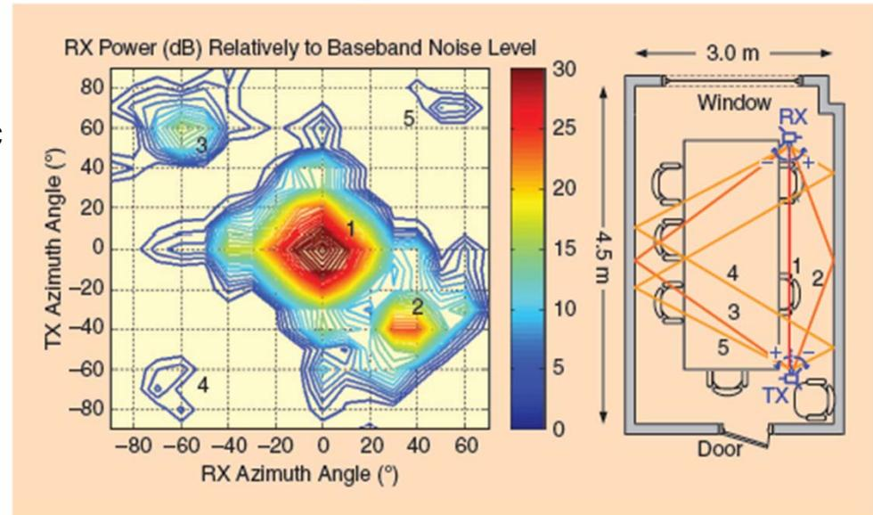
Figure 3. The measured 60 GHz channel in a conference room setting. The measurements clearly show evidence of quasi-optical propagation, e.g., simple to resolve multipath reflections. From [1].
